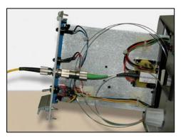
Fig. 1. UGT as sacrificial interface inside instrument.
